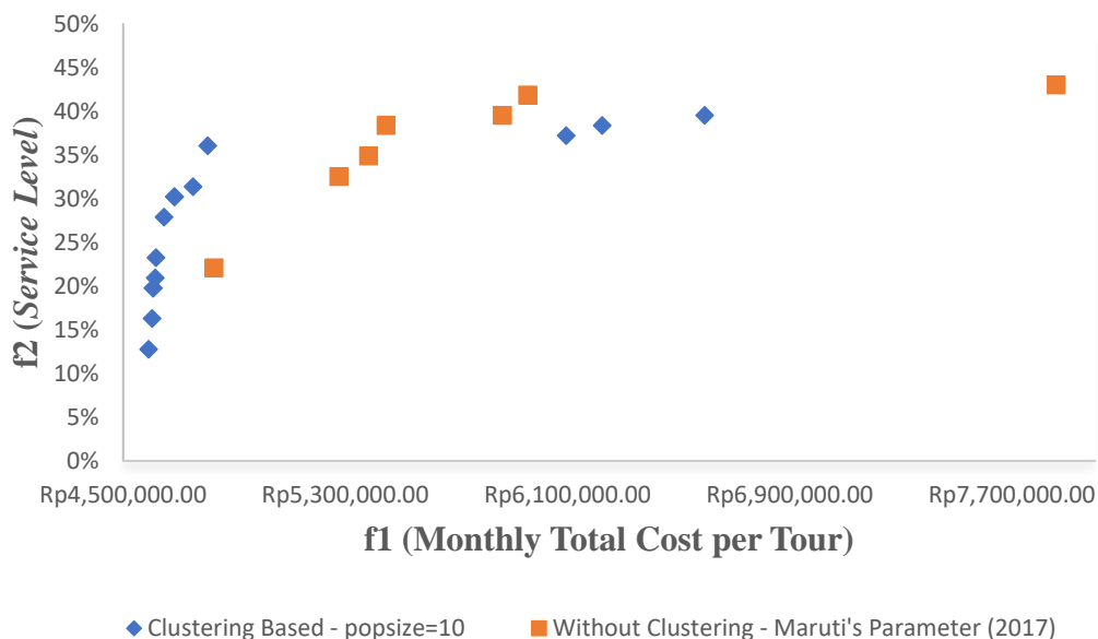
Figure 11. Pareto front of clustering-based NSGA-II with 10 population size vs. NSGA-II with Maruti's (2017) Parameter
